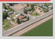
**Phase 4** will reconstruct existing road infrastructure improving safety, and will construct a new grade separation over BNSF railway where none currently exist. This phase will also improve the intersection at SR 97.
